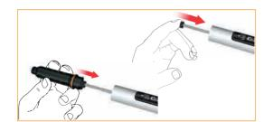
Push the cartridge sleeve into the housing and turn anti-clockwise to lock. You will hear a click.
