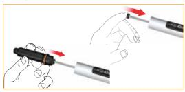
**5** Push the cartridge sleeve into the housing and turn anti-clockwise to lock. You will hear a click.
