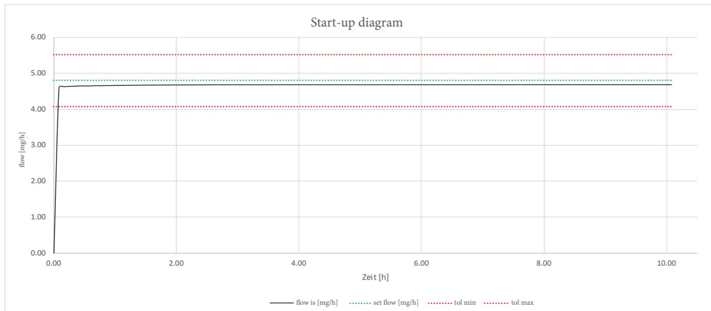
Start-up diagram with delivery rate of 4.8 mg/h
