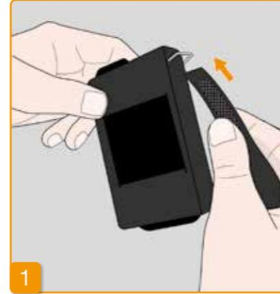
1 Pull both ends of the strap through the hook with each loop side facing outward.
