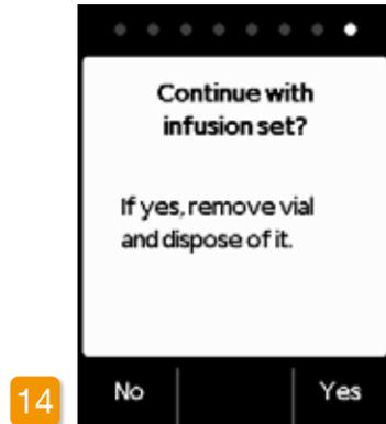
To proceed immediately with the connection of an infusion set, remove the vial and press **Yes**. If you wish to connect the infusion set at a later time, then leave the vial on the pump until that time and press **No**. This will take you to the main screen, where you can then select "Change infusion set" in the menu in [Section 4.3](#) to proceed.
