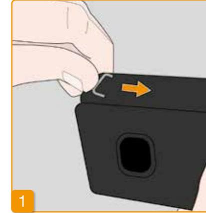
1 Slide the hooks all the way back to prepare the carrier. Protruding hooks could impair carrying comfort.
