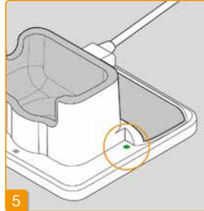
As soon as the spare rechargeable battery is fully charged, the **spare rechargeable battery** signal light will switch from yellow to green.
