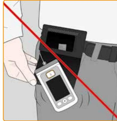
⚠ The opening on the carrying bag should never point downward because the pump could fall out and become damaged.
