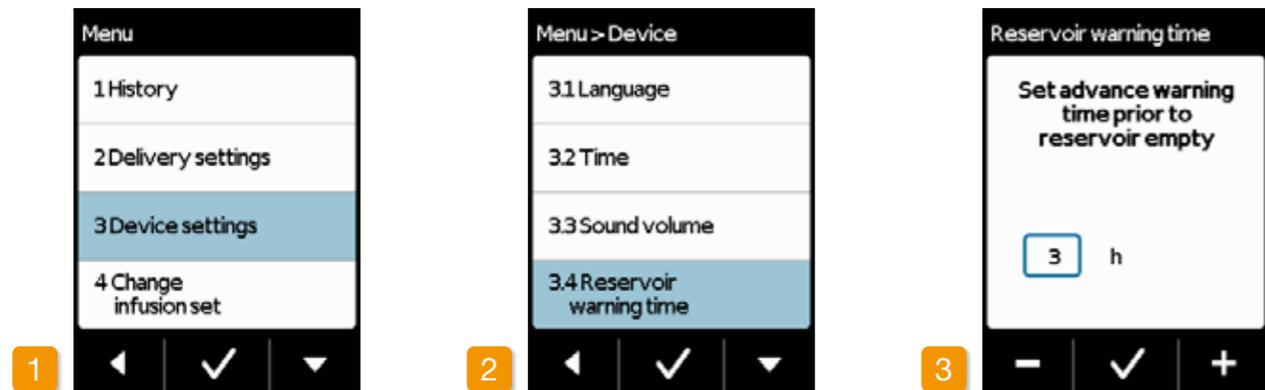
The **Reservoir warning time** function allows you to set the time when your pump will emit the **Reservoir almost empty** warning. The reservoir warning time is the amount of time you have left when the message appears until you have to change the reservoir. This does not take into account the maximum number of boluses.
