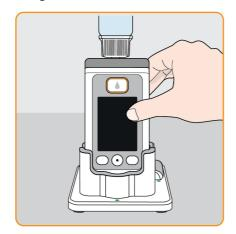
Press to start the filling process. The unit will pump the medication from the vial into the reservoir.
