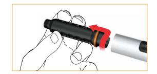
3 Insert the new cartridge into the cartridge sleeve.
