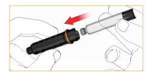
4 Push the threaded rod back completely. This is best performed using your finger tip (but you can also use the new cartridge to push the rod in).
