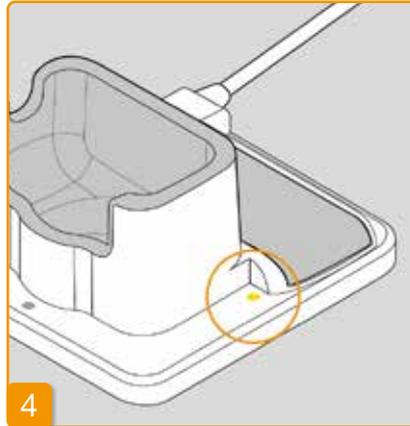
The signal light for the **spare rechargeable battery** will light up yellow. The spare rechargeable battery is charging.
