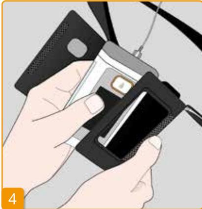
Place the pump in the carrying bag. Make sure that the infusion set is pointing up.
