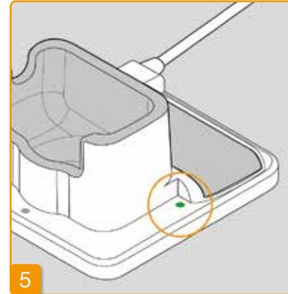
As soon as the spare rechargeable battery is fully charged, the **spare rechargeable battery** signal light will switch from yellow to green.
