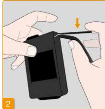
Secure the strap by pressing the hook to the loop side of the strap.
