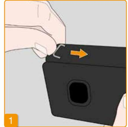
Slide the hooks all the way back to prepare the carrier. Protruding hooks could impair carrying comfort.
