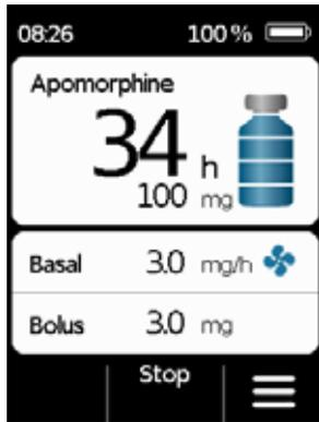
You must stop delivery before you disconnect the infusion set from your body. [Section 3.4](#) Disable the button lock and press **Stop**. Then press
