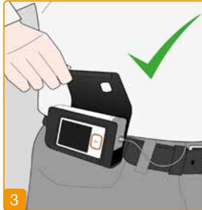
Place the pump in the carrying bag and close the bag. Check to ensure that the infusion set is pointing toward the middle of the abdomen and the opening for pressing the bolus button is completely accessible.
