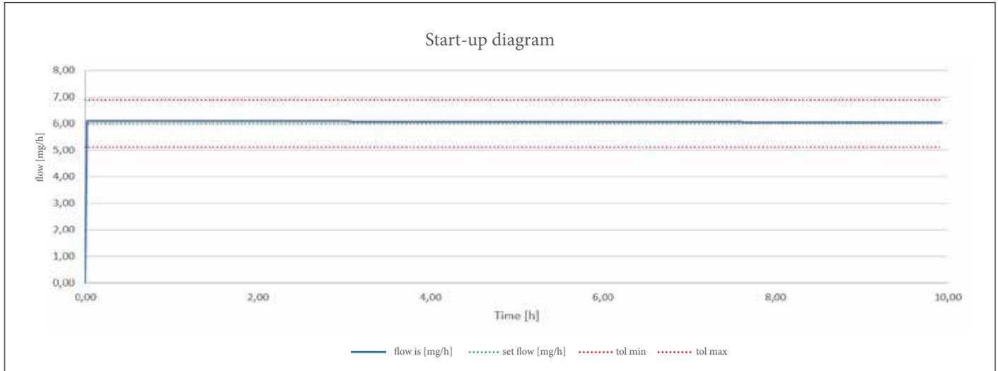
Start-up diagram with delivery rate of 6.0 mg/h
