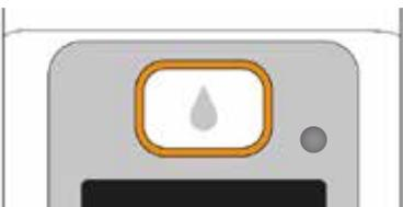
When pressed and released quickly, the bolus button serves as “Home button” and the main screen will be shown.
