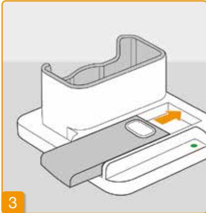
**Insert the spare rechargeable battery into the docking station**
