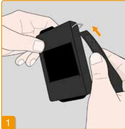
Pull both ends of the strap through the hook with each loop side facing outward.
